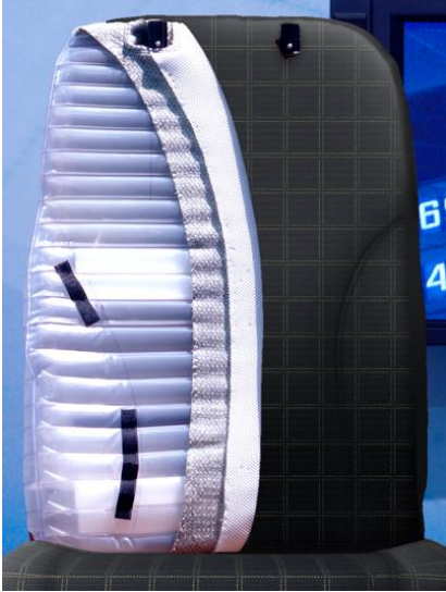
Figure 5: Replacing plastic foam with air cushions saves up to 5 kg of weight per seat. © 2012 Lantal
